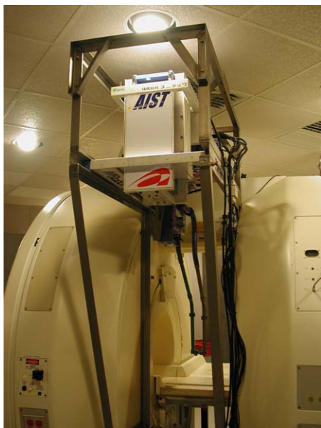
Fig. 3. The robot attached to the open MRI scanner.
